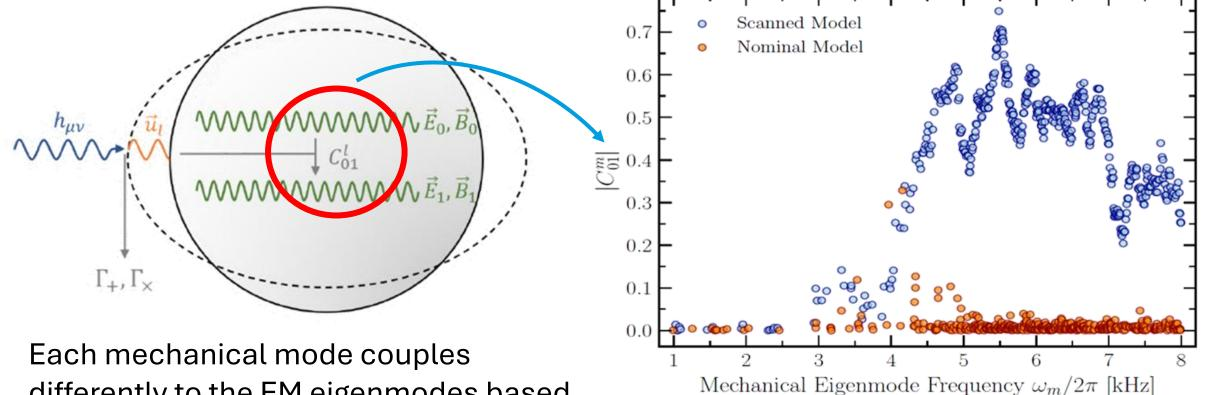
differently to the EM eigenmodes based on the **spatial distribution** of each mode
