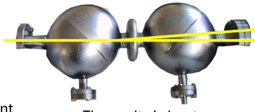
The cavity is bent
