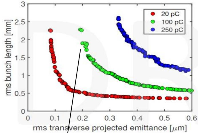
FIG. 6. Results of optimization for various charges for 1  $\mu\text{m}$  / mm thermal emittance.
