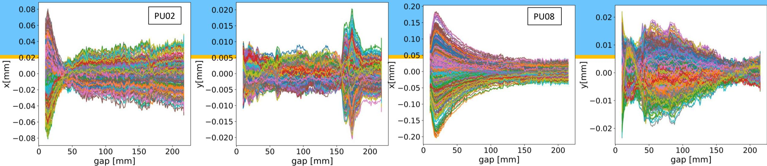
Measurements of the horizontal and vertical orbit were taken varying the gap size in their operation range for 18 IDs in PETRA III. Each colour represents a BPM along the ring.
