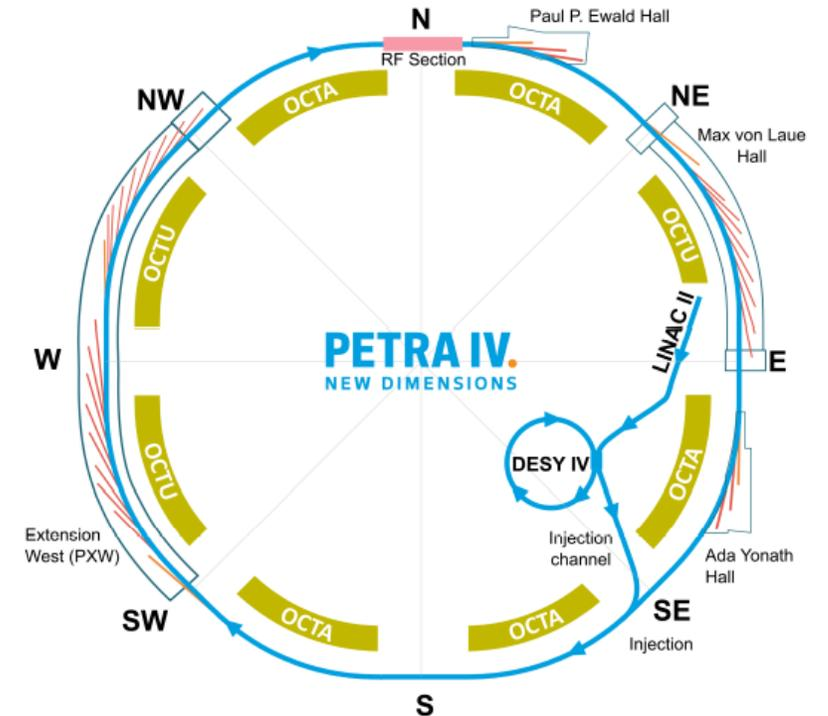
The storage ring will feed up to **30 undulator** insertions (photon beam can be further split to allow more experimental stations).
