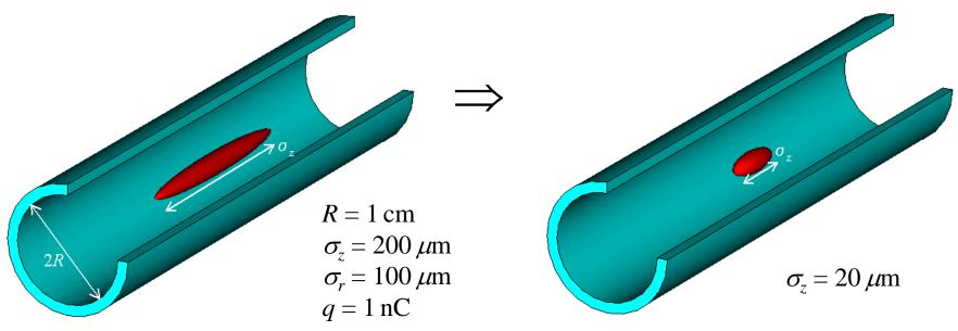
field energy =  $W_{tot} = 0.107 \text{ mJ}$   $\Delta W_{tot} = 0.958 \text{ mJ}$   $W_{tot} = 1.065 \text{ mJ}$ CSR in the last arc of Zeuthen benchmark BC (steady state assumption):  $R_0 = 10 \text{ m}, \ \sigma_z = 20 \ \mu \text{m}, \ L = 0.5 \text{ m} \rightarrow P = 375 \text{ kW}, \ P \ L/c_0 = 0.625 \text{ mJ}$
